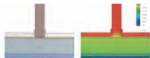
Fig. 4. Development of isotherms for a KLH wall on a concrete floor slab with external insulation at the same time. It can be clearly recognised that the KLH panel is no longer intersected by the 10° and 12° isotherms (mould and condensation isotherms limit).
